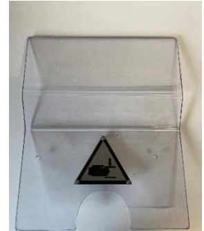
B-1018: Security shield by inlet of fish
