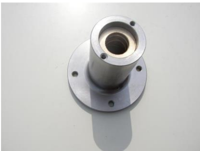
B-1031: House and bearing complete for bushmotor
