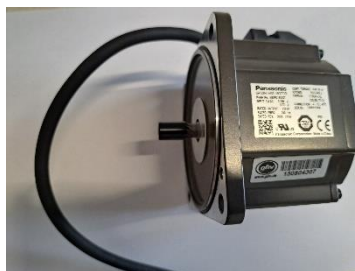
SB-107: Panasonic brushless motor for round knife
