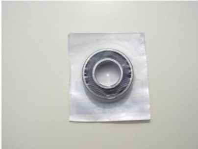
K-1041: Bearing \varnothing 35/\varnothing 17 (shaft for chain)
