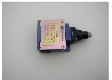
K-1046: micro switch (for gate) (old model)
