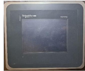
SB-105: Display for controle box
