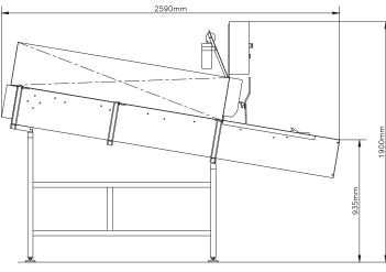
Compressed air: Air Compressor: Power: Water consump.: Weight: Material: min. 6 bar min. 2 KW 380v, 50Hz (or other) 500 l/h, adjustable 350 Kg AISI 304 Stainless steel
