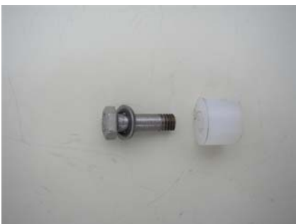
K-1055: Roll with shaft (slitting element)
